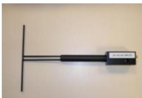
Figure 1 – Satimo COMOSAR Validation Dipole
